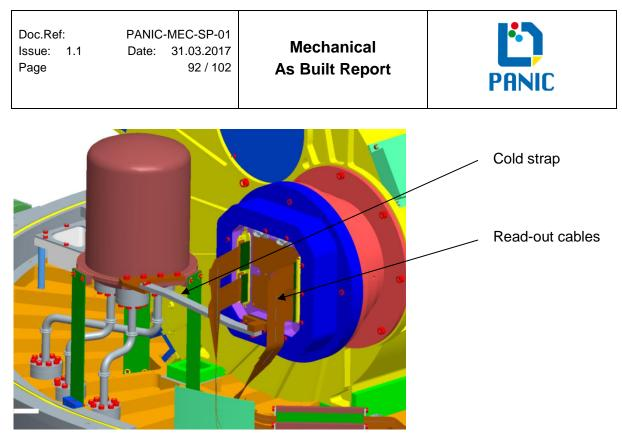
Figure 73: Detector assembly
