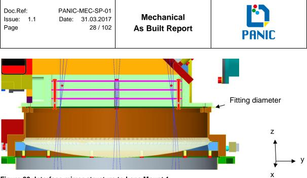
Figure 20: Interface mirror structure to Lens Mount 1
