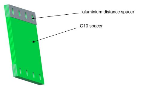
Figure 55: Stack of G10 spacers. Four spacers form a stack at PANIC
