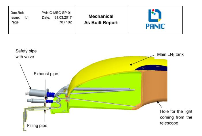
Figure 51: Cross section through the main tank showing the connecting pipes
