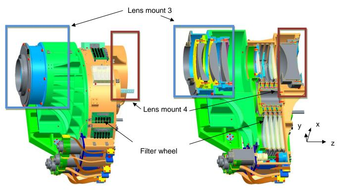
Figure 33: Optics mount 2 and its components
