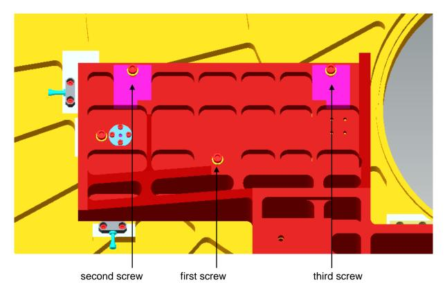
Figure 32: Sequence to tighten the screws of Cold Stop Wheel
