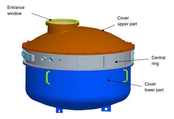
Figure 48: The vacuum vessel.
