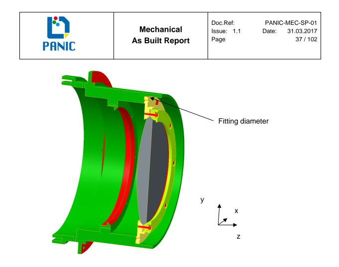
Figure 29: Lens 5 with its support in Lens Mount 2
