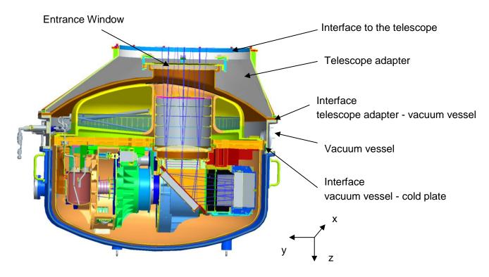
Figure 11: Interfaces and components included in "complete optics"
