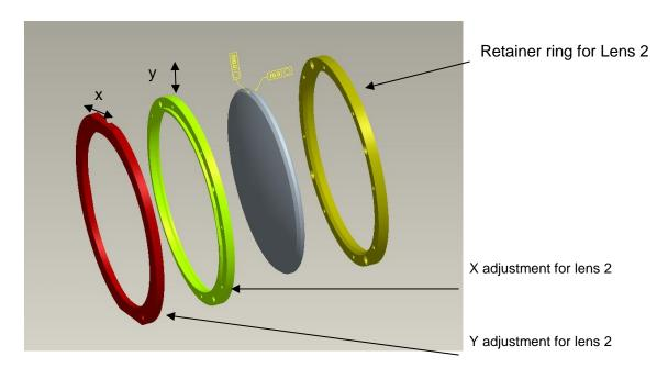
Figure 27: Adjustment unit for Lens 2
