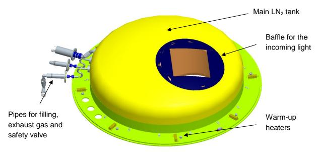
Figure 50: The main tank subassembly
