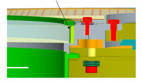
The inner diameter of this ring is large enough to ensure a gap to the filters of 0.5mm at cold. Assuming the FSi substrate does not shrink at all and remains at 117.855 mm in diameter, the inner diameter of the ring has a diameter of 119.4 mm at warm resulting in 118.95 mm at cold. The resulting gap will be 0.55 mm.
