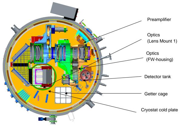
Figure 59: Distribution of the temperature sensors inside the PANIC cryostat. Not shown are the sensors on the  $LN_2$  main tank, on the shield and inside the detector module.
