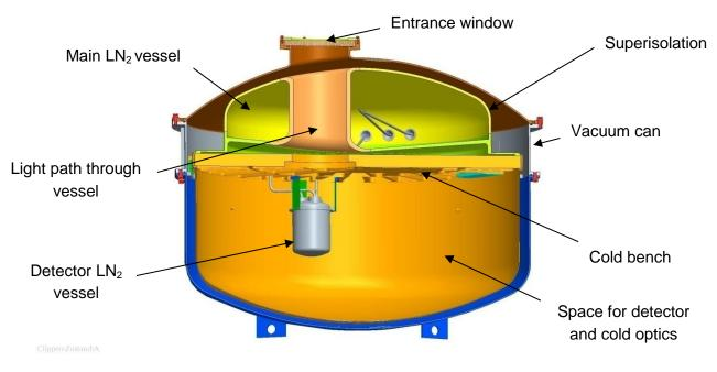
Figure 47: cross section through the cryostat
