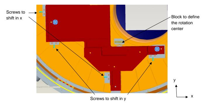
Figure 17: Optics mount 1 adjustment principle
