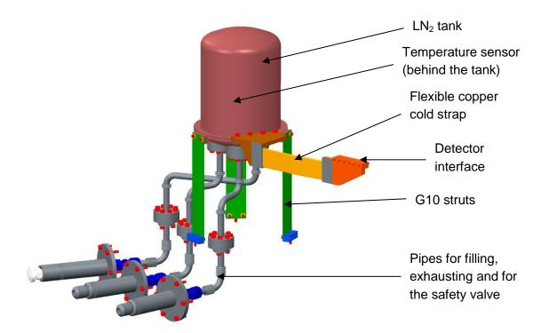
Figure 53: The detector tank subassembly
