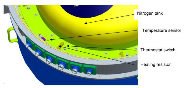
Figure 60: Eight heaters in two circuits attached to the nitrogen tank are used to warm-up PANIC
