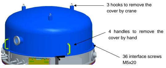
Figure 62: removing the vacuum cover
