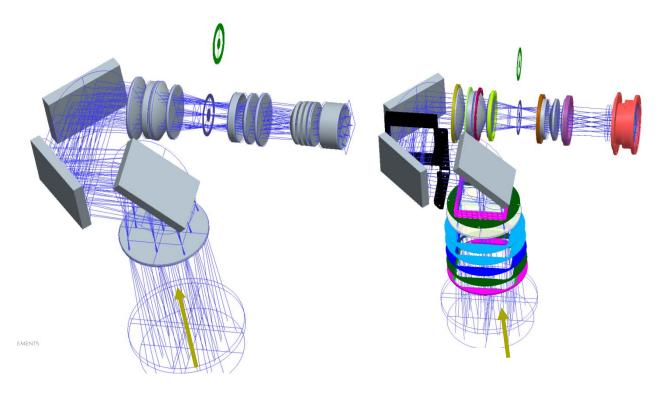
Figure 7: The optical layout with lenses and mirrors(left) and with baffles (right)
