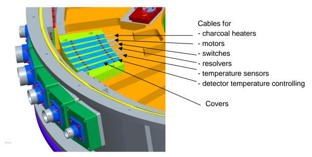
Figure 57: Feedthroughs for the cryostat cabling
