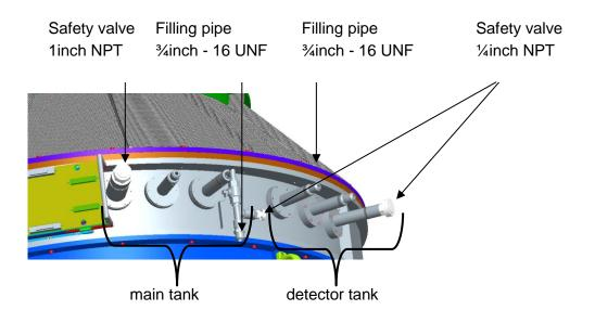
Figure 65: Connections to the tanks for the cryogenic liquids
