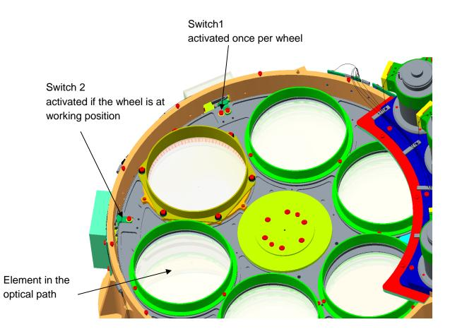
Figure 45: Two switches per wheel provide information about the actual wheel position
