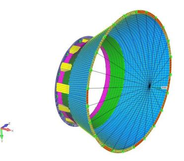
Figure 68: FE-Model of the telescope adapter
