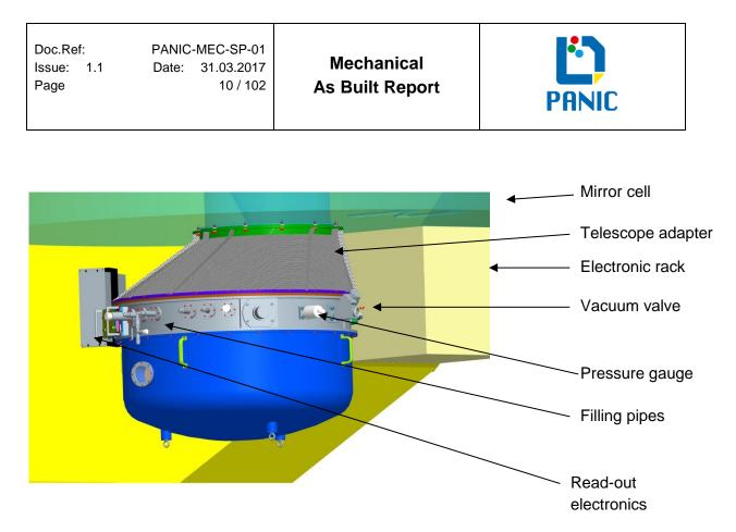
Figure 3: PANIC at the 2.2m telescope
