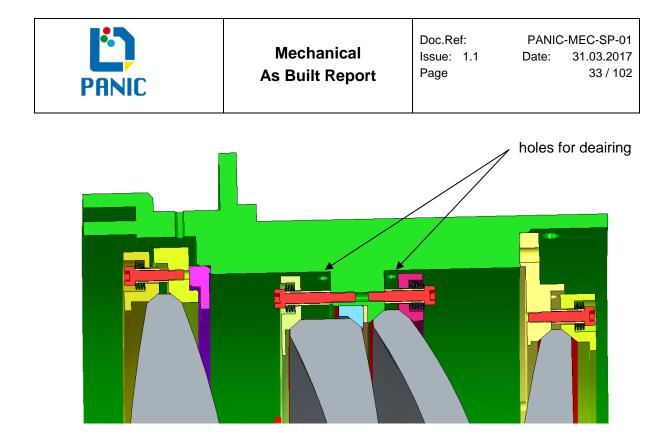
Figure 25: De-airing is done by radial holes
