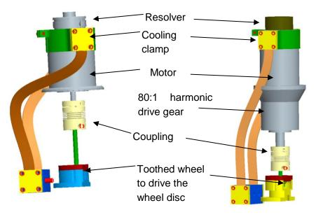
Figure 44: The main parts of the wheel drives. Left: one of four identical filter wheel power trains, right: the power train for the cold stop wheel
