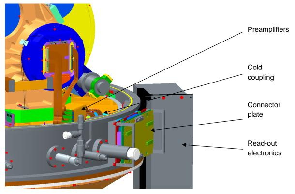
Figure 74:Read-out cabling
