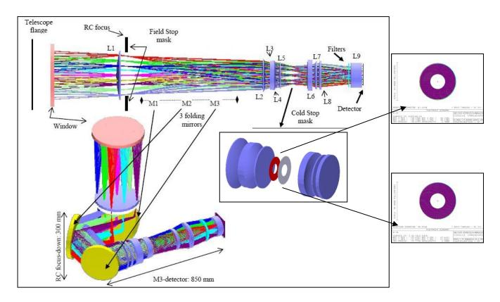
Figure 4: PANIC optical layout, original (top) and folded (bottom)
