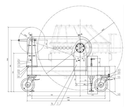
Figure 76: Dimensions of trolley A
