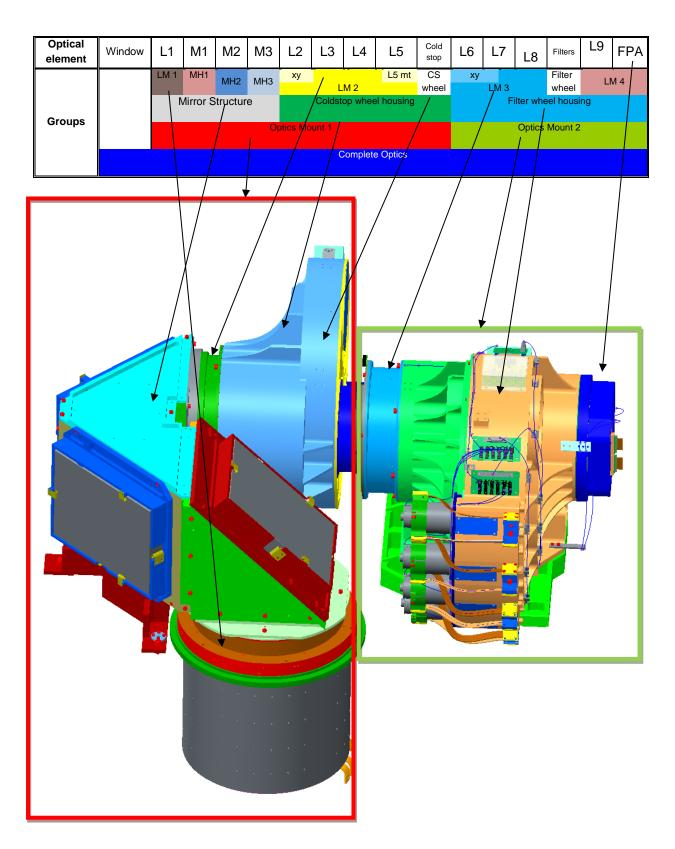
Figure 8: Overview over the optical elements and their mounts
