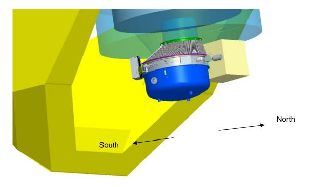
Figure 66: Orientation of PANIC at the 2.2 m telescope
