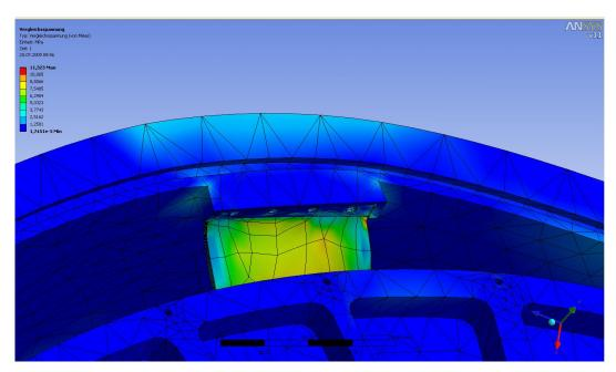
Figure 56: Finite element simulation of the spacers
