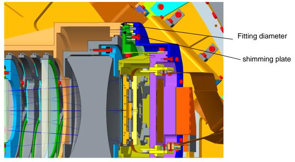
Figure 42: The interface to the detector
