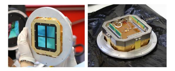
Figure 5: The focal plane array. The greenish areas are the 4 light sensitive areas (left). The back of the module with connectors and heaters (right)
