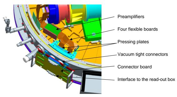
Figure 58: Feedthroughs for the detector read-out.
