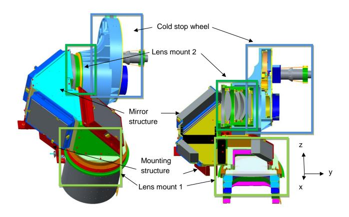
Figure 14: Optics mount 1 and its sub-components
