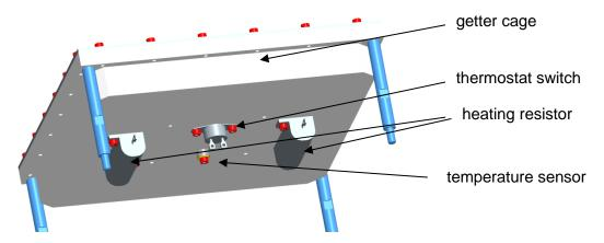
Figure 61: Two heaters, a thermostat switch and a temperature sensor are used to control the temperature of the getter cage
