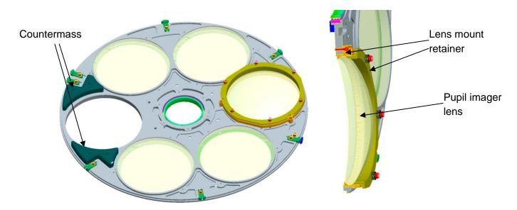
Figure 38: Filter wheel 1 with the pupil imager lens and counterweights
