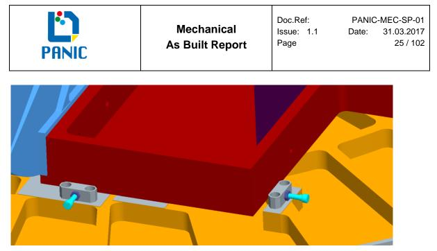
Figure 16: Adjustment screws allow optics mount 1 to be shifted in x and y direction.
