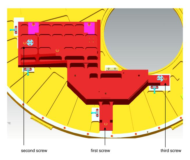
Figure 18: Sequence to tighten the screws of OM1
