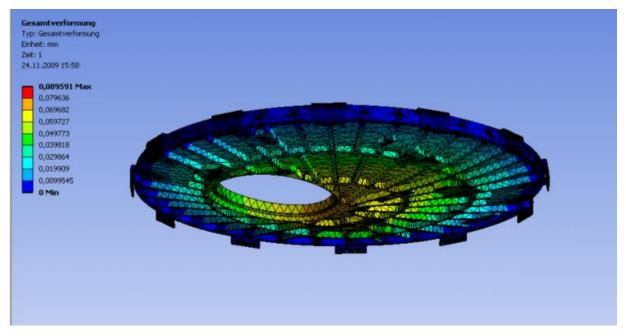
Figure 13: Results of the simulation with different orientations. top: telescope pointing to horizon, bottom: telescope pointing to zenith
