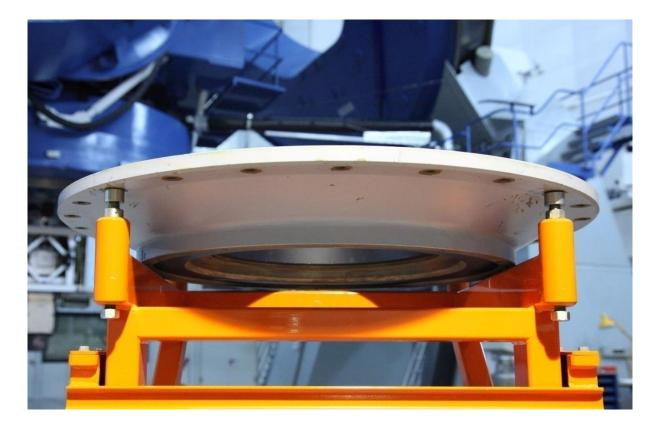
Figure 69: An adapter flange allows instruments designed for the 2.2 m telescope to be used at the 3.5 m telescope
