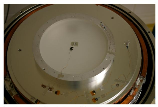
Figure 12: Test set-up for Thermal cycling test with lens 1 dummy.
