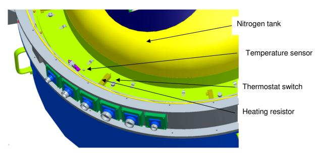
Figure 58: Eight heaters in two circuits attached to the nitrogen tank are used to warm-up PANIC
