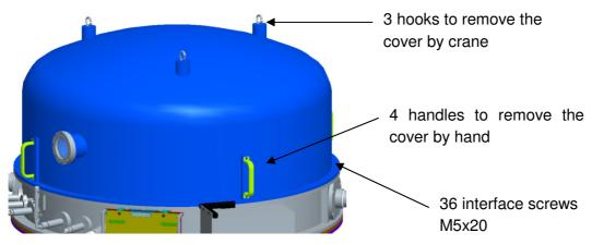
Figure 60: removing the vacuum cover
