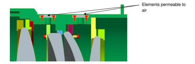
Figure 25: Deairing is done by sintered aluminum elements which are permeable to air
