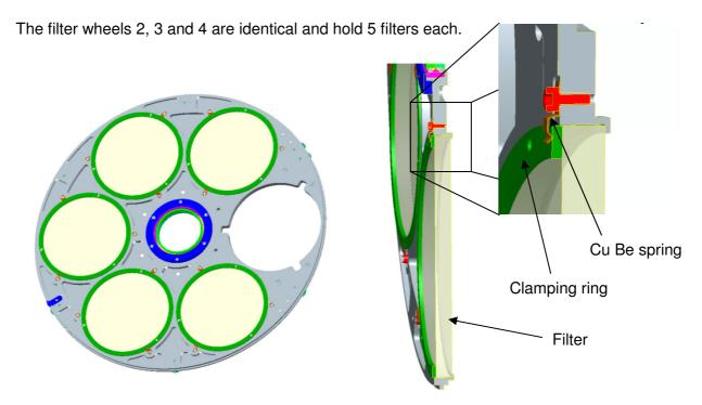
Figure 36: Left: Design of the filter wheels 2 - 4. Right: Cross section showing mounting concept.
