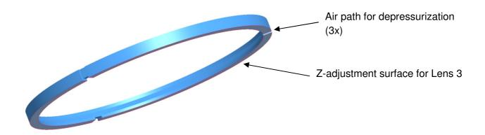
Figure 28: Adjustment ring for lens 3
