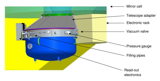
Figure 5: PANIC at the 2.2m telescope
