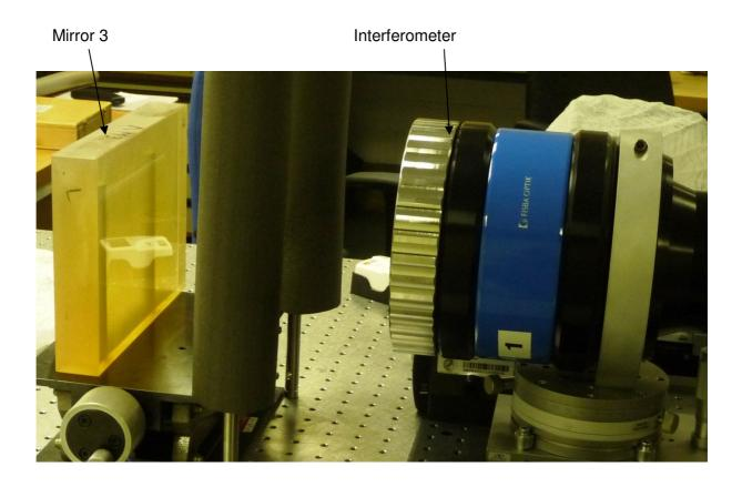
Figure 80: The uncoated mirror 3 is tested with an interferometer before integration into its mount.
