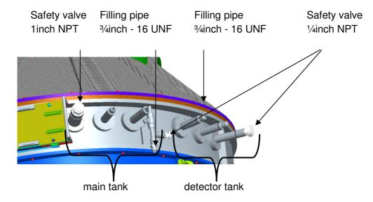
Figure 63: Connections to the tanks for the cryogenic liquids
