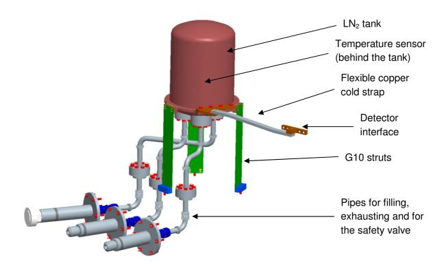
Figure 51: The detector tank subassembly
