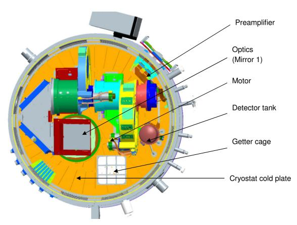
Figure 57: Distribution of the temperature sensors inside the PANIC cryostat. Not shown are the sensors on the  $LN_2$  main tank, on the shield and inside the detector module.
