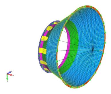
Figure 66: FE-Model of the telescope adapter
