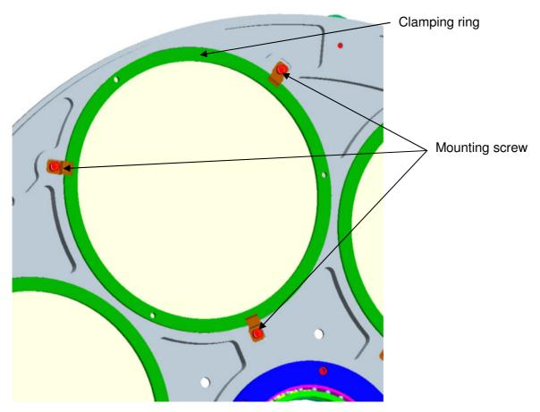
Figure 38: Filter mounting elements
