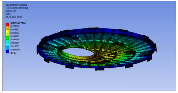
Figure 15: Results of the simulation with different orientations. top: telescope pointing to horizon, bottom: telescope pointing to zenith
