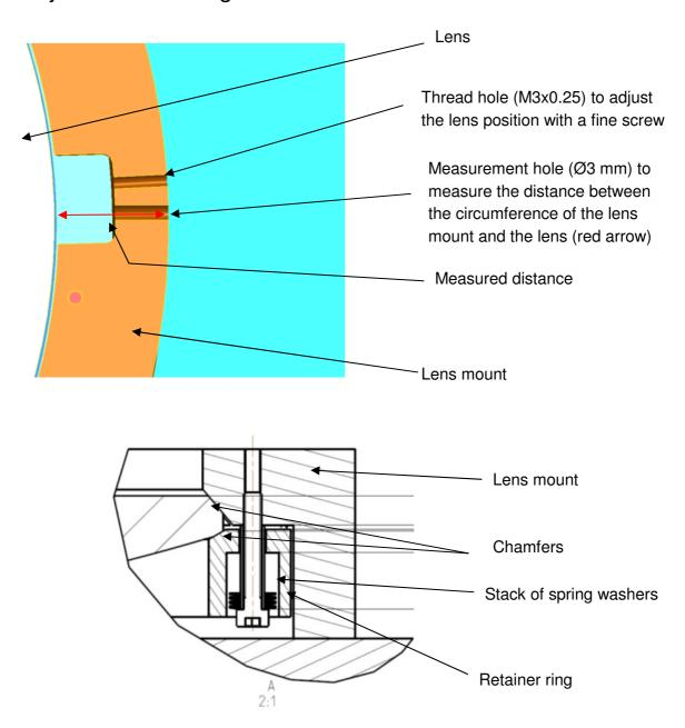
Figure 10: Cross-sectional view through the lens alignment design (explanation in the text)
