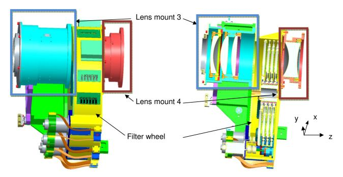
Figure 31: Optics mount 2 and its components
