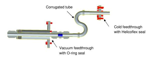
Figure 50: Cross section through the exhaust pipe
