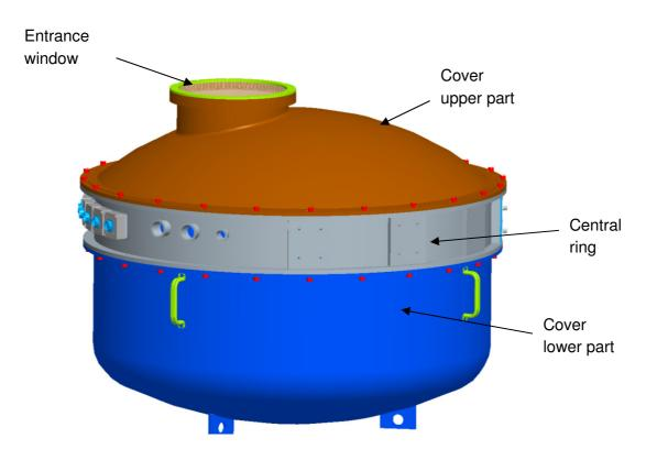
Figure 46: The vacuum vessel.
