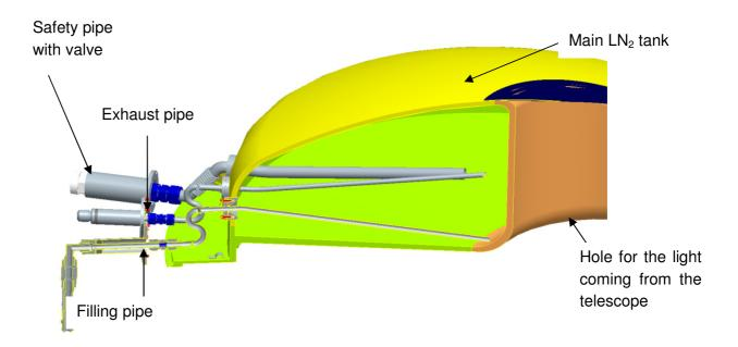
Figure 49: Cross section through the main tank showing the connecting pipes
