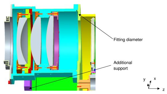
Figure 33: Positioning of lens mount 3
