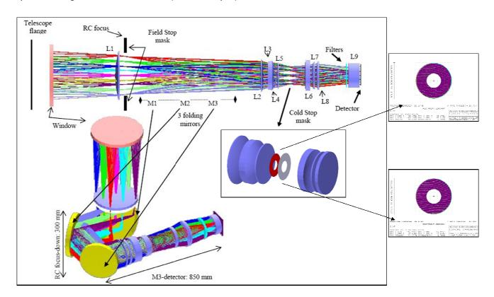
Figure 2: PANIC optical layout, original (top) and folded (bottom)
