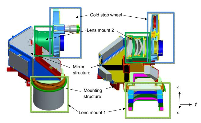
Figure 16: Optics mount 1 and its sub-components
