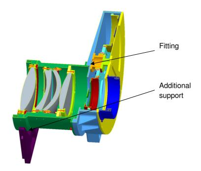
Figure 26: Positioning of lens mount 2
