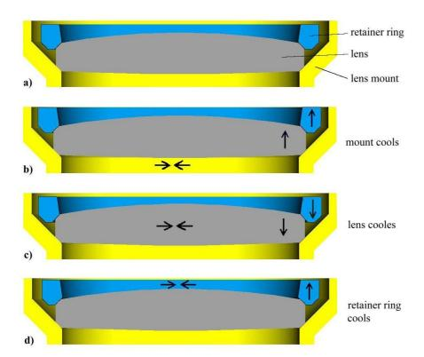
Figure 11: Displacements of lens and retainer ring due to thermal shrinkage while cooling down (explanation in the text)
