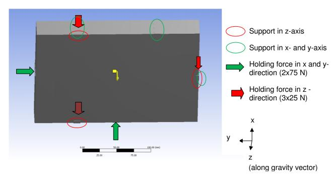
Figure 23: Boundary conditions to model the mirror support
