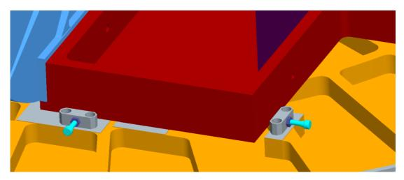
Figure 17: Adjustment screws allow optics mount 1 to be shifted in x and y direction.
