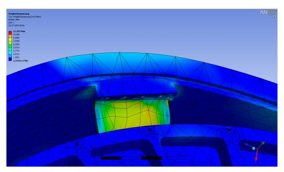
Figure 54: Finite element simulation of the spacers
