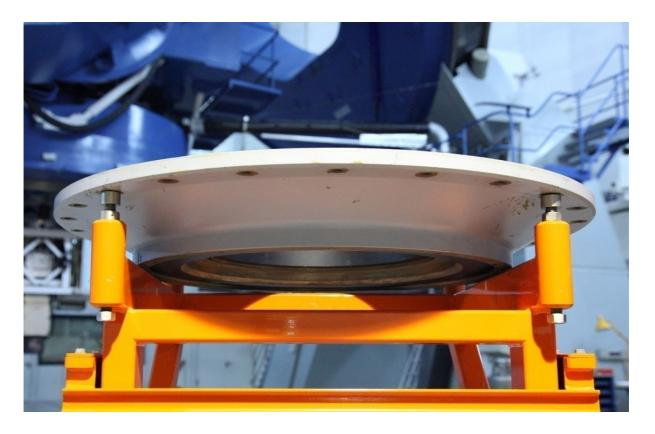
Figure 67: An adapter flange allows instruments designed for the 2.2 m telescope to be used at the 3.5 m telescope
