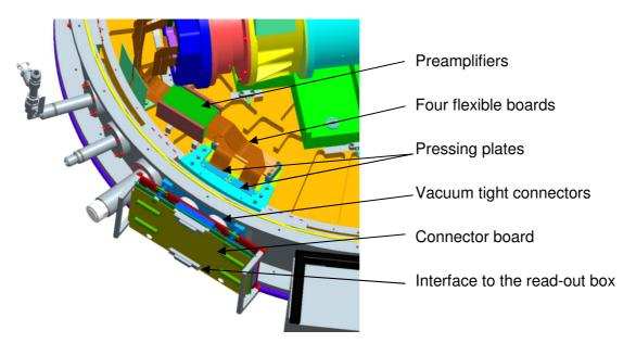
Figure 56: Feedthroughs for the detector read-out.
