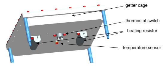
Figure 59: Two heaters, a thermostat switch and a temperature sensor are used to control the temperature of the getter cage
