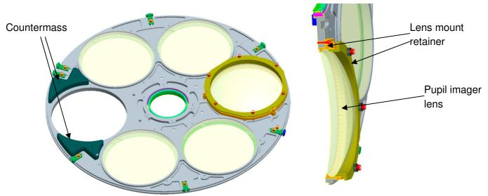
Figure 35: Filter wheel 1 with the pupil imager lens and counterweights
