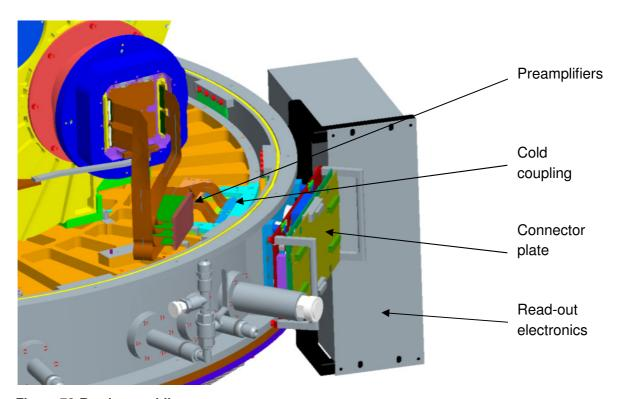
Figure 72:Read-out cabling
