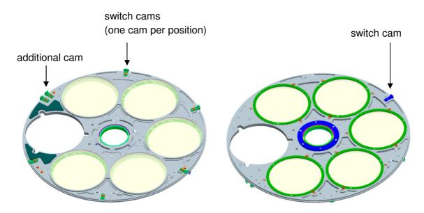
Figure 44: The filter wheel disc front side (left) has one cam per position, the rear side (right) has only one cam.
