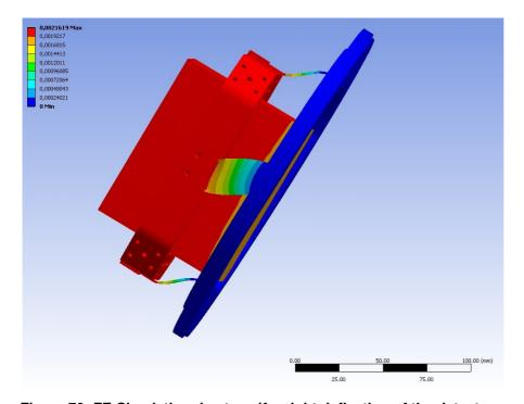
Figure 70: FE-Simulation due to self weight deflection of the detector mount
