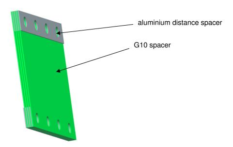
Figure 53: Stack of G10 spacers. Four spacers form a stack at PANIC
