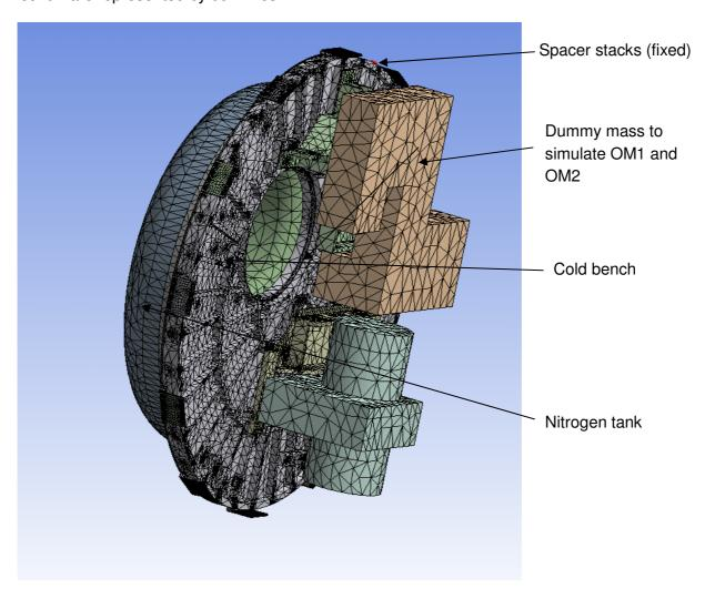
Figure 14: Simulation of the cold bench including the dummy masses.
