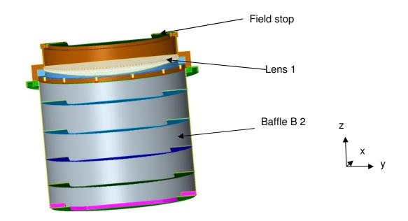
Figure 19: Lens mount 1 with lens 1, the field stop and the baffle B2
