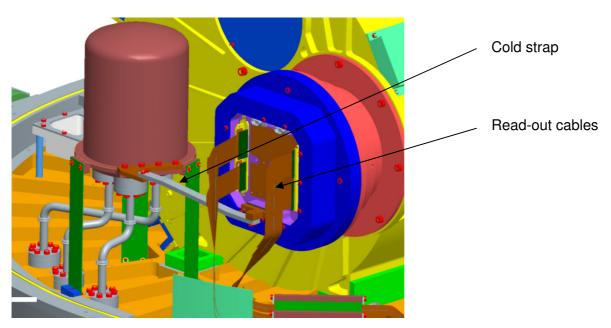
Figure 71: Detector assembly
