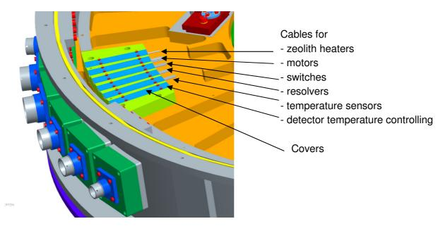
Figure 55: Feedthroughs for the cryostat cabling
