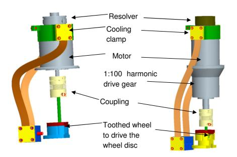
Figure 42: The main parts of the wheel drives. Left: one of four identical filter wheel power trains, right: the power train for the cold stop wheel
