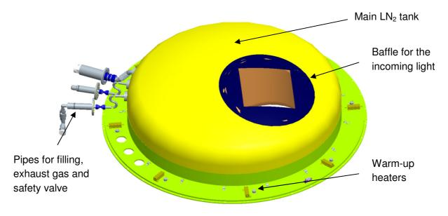
Figure 48: The main tank subassembly
