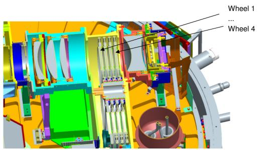
Figure 34: The wheels are numbered according to their order in the light-path
