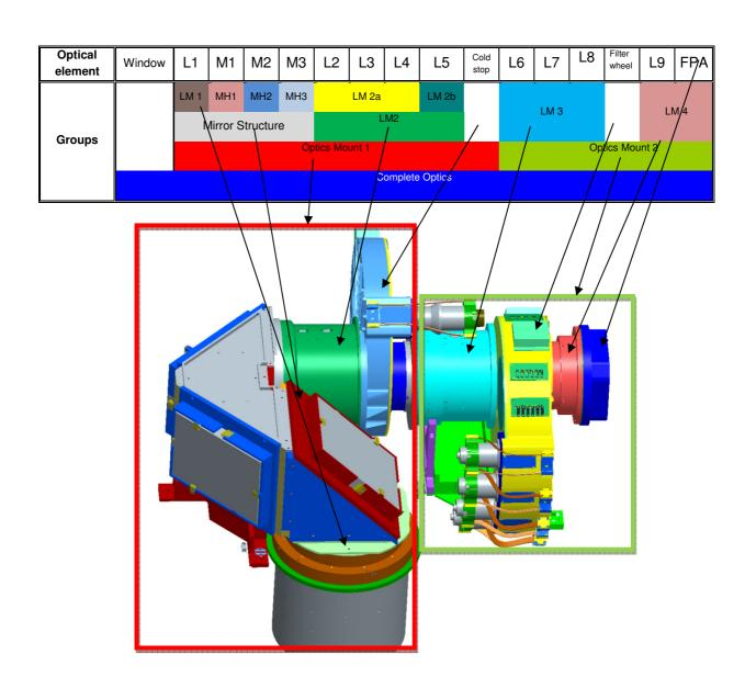
Figure 9: Overview over the optical elements and their mounts
