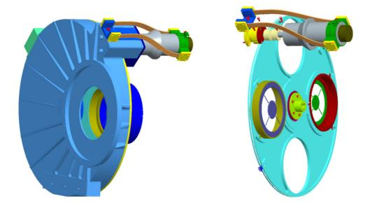
Figure 30: The cold stop wheel; left the complete view right without cover
