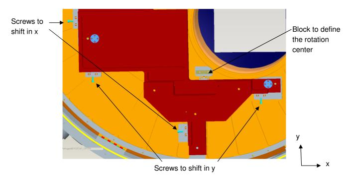
Figure 18: Optics mount 1 adjustment principle
