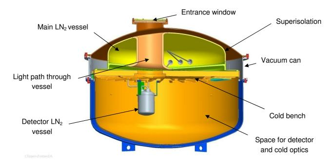
Figure 45: cross section through the cryostat
