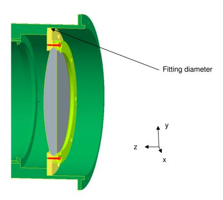
Figure 29: Lens 5 with its support in lens mount 2
