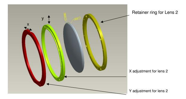
Figure 27: Adjustment unit for Lens 2
