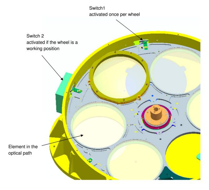
Figure 43: Two switches per wheel provide information about the actual wheel position
