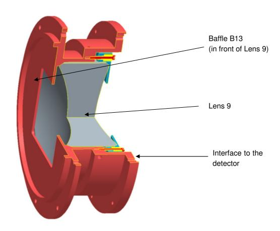
Figure 39: Lens mount 4 with lens 9 attached.
