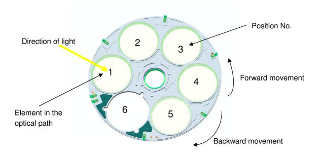
Figure 41: Definition of wheel positions and directions
