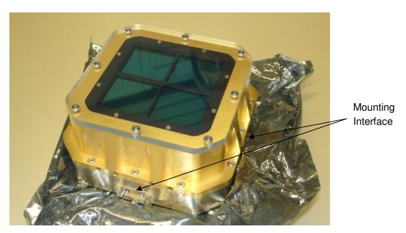
Figure 68: The detector module as delivered from Teledyne
