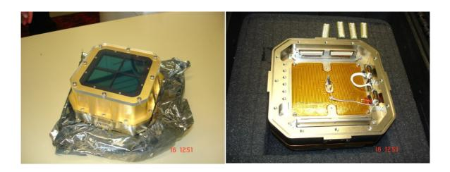
Figure 3: The focal plane array. The greenish areas are the 4 light sensitive areas (left). The back of the module with connectors and heaters (right)
