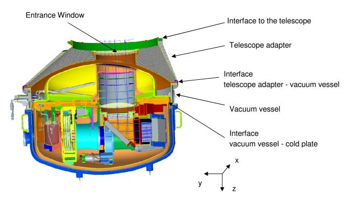
Figure 13: Interfaces and components included in "complete optics"
