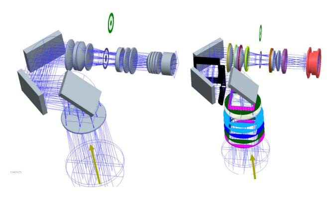
Figure 8: The optical layout with lenses and mirrors(left) and with baffles (right)
