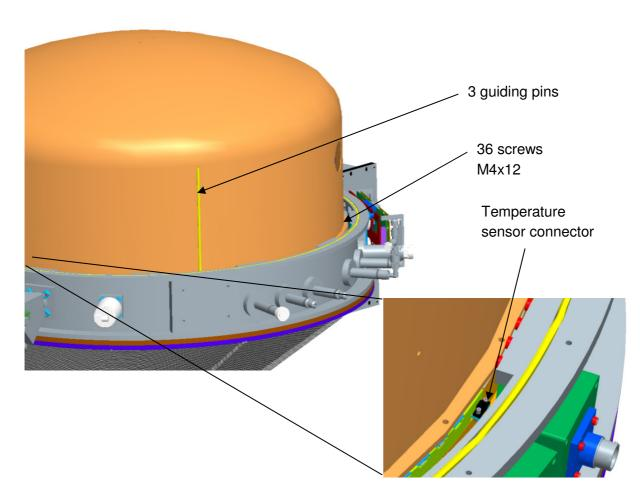
Figure 61: removing the nitrogen shield
