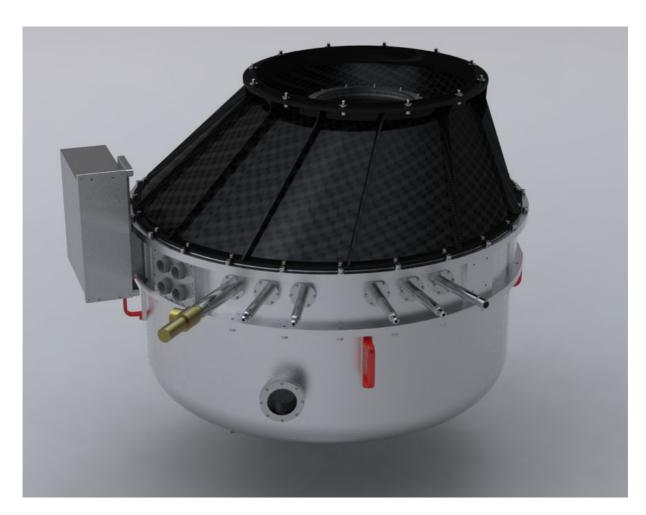
Figure 1: Artificial view of the cryostat with filling pipes, read-out electronics and the conical telescope adapter
