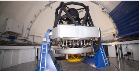
Left: J-PAS 2.5m telescope installed at Pico del Buitre, in Javalambre Observatory. Right: JPCam, the J-PAS camera, a 3D model showing the 14 CCDs and the cryogenic dewar.
