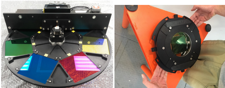
FIGURE 2.3 Left: One of the T8oSCam filter wheels with the filters mounted on it. It represents one of the two wheels marked in red in Fig. 2.2. Right: A picture of the camera showing the CCD before being mounted on the telescope.
