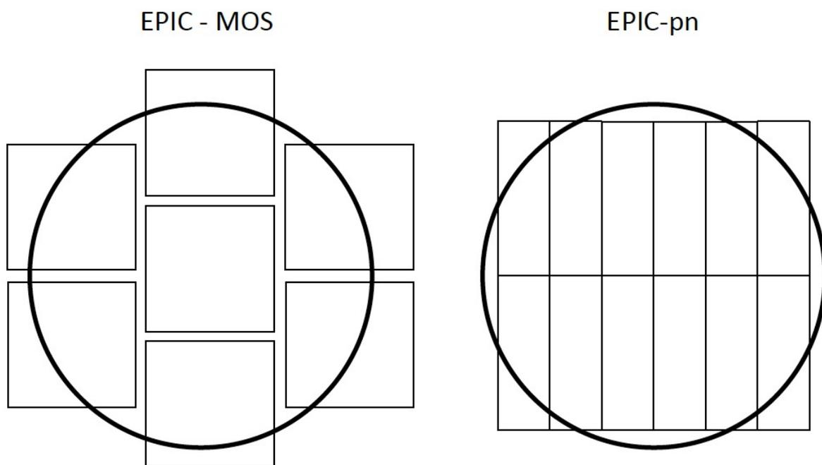
**Figure 1.10: EPIC detector on board *XMM-Newton* satellite** - The EPIC-MOS cameras are composed by seven CCDs each of  $10.9 \times 10.9$  arcmin; the EPIC-pn camera is composed by 12 CCDs each of  $13.6 \times 4.4$  arcmin. The circle diameter corresponds to 30 arcmin – Image courtesy of Dr. Toalá.
