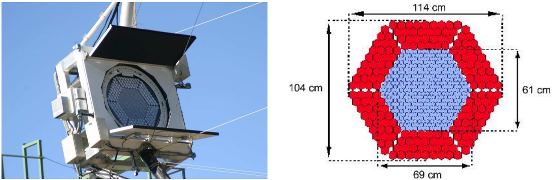
Figure 7.3 Left : The MAGIC camera with the lids opened. The hexagonal shape, composed by 577 PMTs, is clearly seen in the picture. Right : Pixel scheme of the camera, with 397 1" inner pixels (blue) and 180 1.5" outer pixels (red). The total FoV is 3.5^\circ \times 3.8^\circ .
