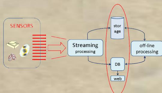
Figure 2. Schematic view of TarGet infrastructure used in LOFAR telescope for sensor network data streaming processing and off-line processing. <http://www.rug.nl/target>
